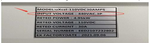
2. After confirming that the input voltage is correct, connect the input power cord to the input terminal of the charger.
