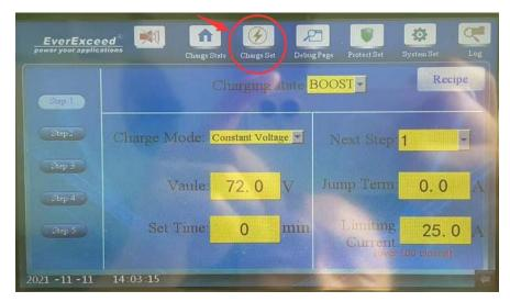
8. Click the start button on the touch screen to start the charger, measure the output voltage with a multimeter, and observe whether the charging voltage rises slowly. If it rises slowly, there is no problem. If it rises suddenly, it is recommended to change the phase sequence of the input three-phase power before starting.
